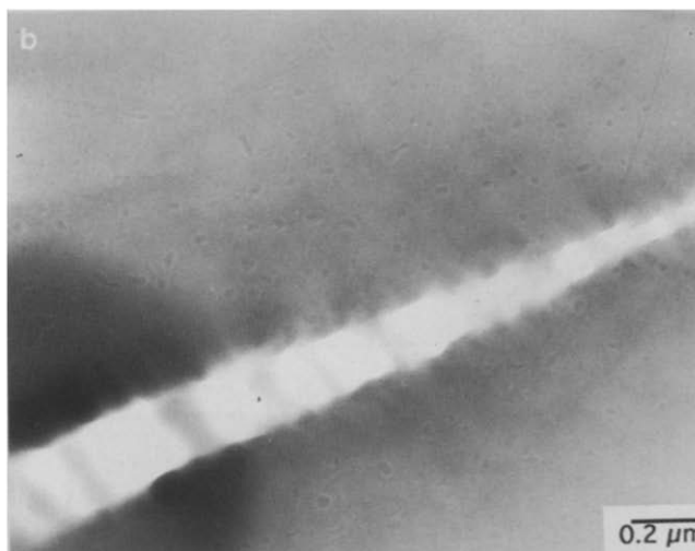
Figure 11 TEM micrographs of PC (a) directly in front of fatigue crack tip demonstrating fibril breakdown; and (b) the region further out in front of the fatigue crack, where there is evidence of crazing with fibrils still intact
